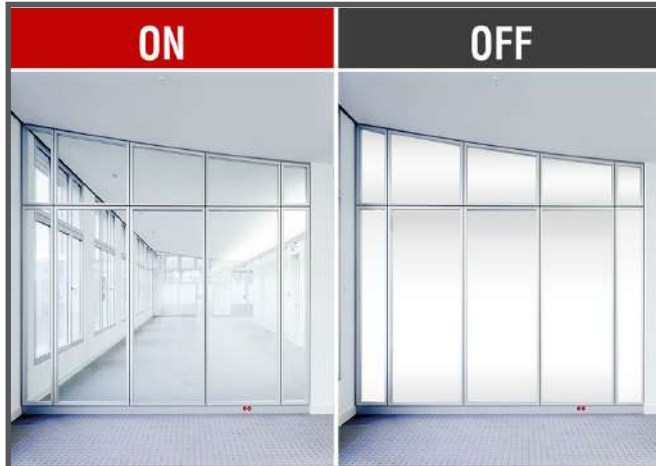
Milky White, High Transparency Light Transmittance: On- 83%; Off- 2%
